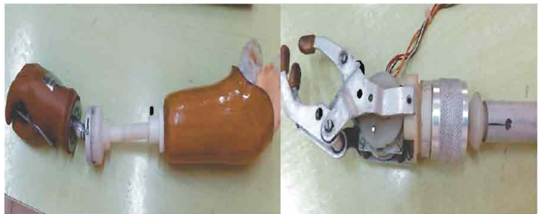
This unit is also, in the process of developing Electric hand with multiaxial wrist unit that will help the user to lock the terminal device (Electric hand) in desired position.
