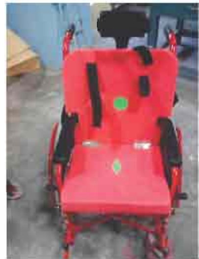
Customization of wheelchair with detachable postural control device
